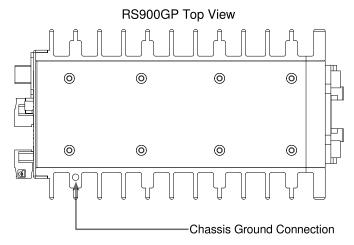
Figure 2.6. RS900GP Chassis Ground Connection
